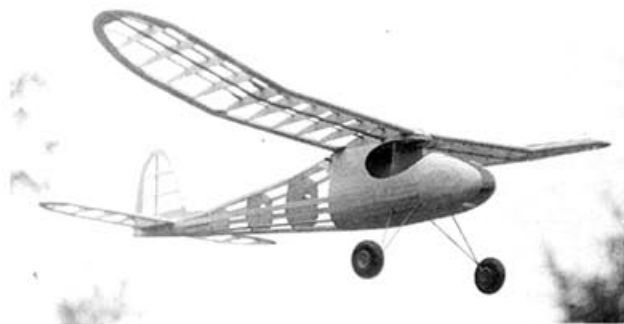
A multi-stringer fuselage built on a crutch is a feature of this 45 in. free-flight power model by the author.
