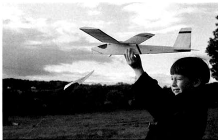
The glider version about to be towed up. Note tissue pennant on towline and slight nose-up angle of model.
