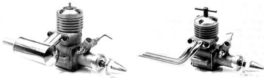
These pictures show virtually the same engine design except that that on the left uses a glowplug and that on the right is a diesel — note the difference in the cylinder heads. The glow engine also has a simple cylindrical silencer rather than a 'straight-through' exhaust.
