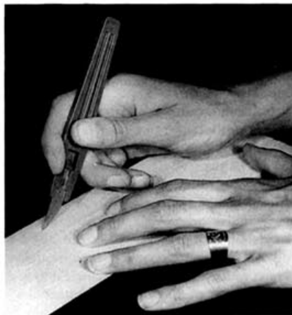
A basic tool is a sharp modelling knife or surgical scalpel. Remember not to use excessive force and that blunt blades lead to accidents.
