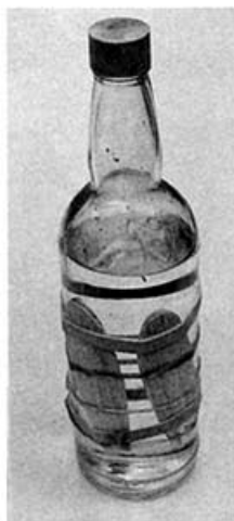
The propeller blades rubber-banded to a suitable diameter bottle.
