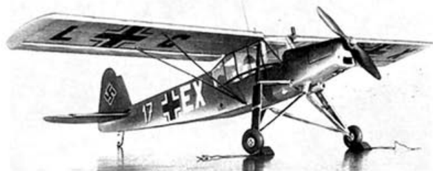
A free-flight model Fieseler Storch, an example of the high-wing layout most successful for F/F models.
